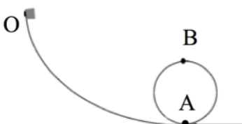
Figure 1. Diagram of roller-coaster track in tutorial problem. Students are asked, “A cart is released at point O, goes down a hill, and goes around a vertical loop in the track. What forces act on the cart when it is at point B?”
